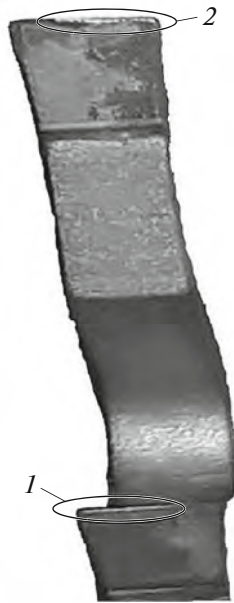
Fig. 1. Flank wear of two adjacent teeth of a circular saw blade after milling grooves in chipboard ( \times 10 ): (1) and (2) adjacent teeth with a limited wear zone.
