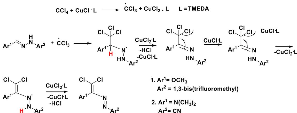
Scheme 2. The mechanism of considered reactions in the quantum chemical calculations.
