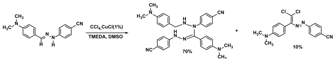
Scheme 6. General scheme of the reaction involving ((E)-4-(2-(4-(dimethylamino)benzylidene)hydrazinyl) benzonitrile.
