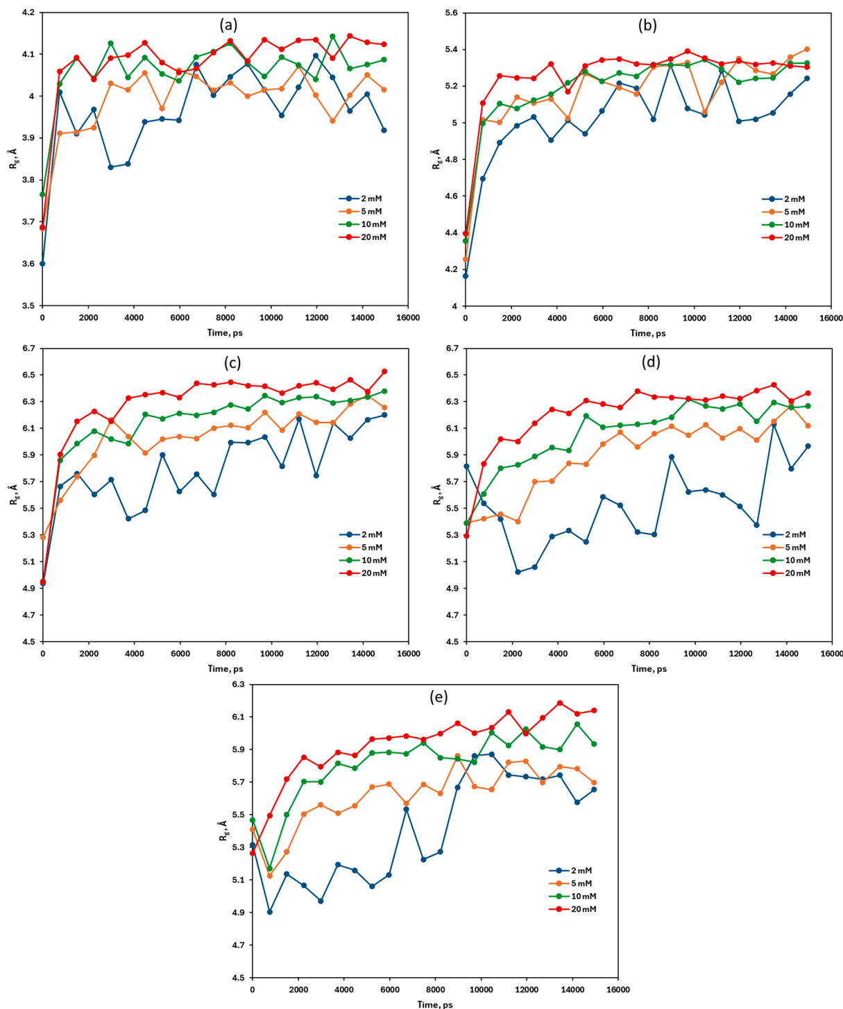
Fig. 7. Radius of gyration evolution of carboxylate groups of pseudo-gemini surfactants at different concentrations for (a) C_{10} -PiPO 2 -C 10 , (b) C_{14} -PiPO 2 -C 14 , (c) C_{18} -PiPO 2 -C 18 , (d) C_{18:1} -PiPO 2 -C 18:1 , (e) C_{18:3} -PiPO 2 -C 18:3 .
