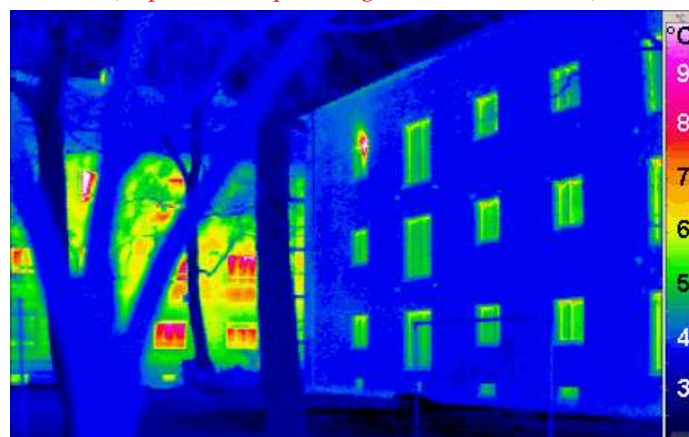
Fig 9. Passive house thermal difference with conventional one in a cold winter days
