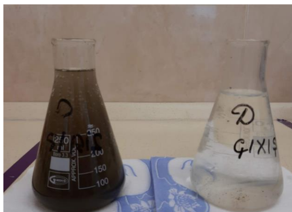
Figure 2. Industrial wastewater sample from entry and exit pit
